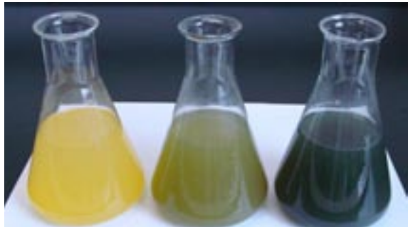
Figure 3 Freshly squeezed orange juice. Left flask: before the endpoint, the colour of the solution reflects the bright orange colour of fresh orange juice and is unaffected by addition of iodine. Centre flask: Once all the ascorbic acid has been oxidised, a slight excess of added iodine complexes with the starch indicator, giving the solution a green colour in this case. This is the endpoint of the titration. Right flask: If further iodine solution were to be added, the solution's green colour would become darker as shown.
