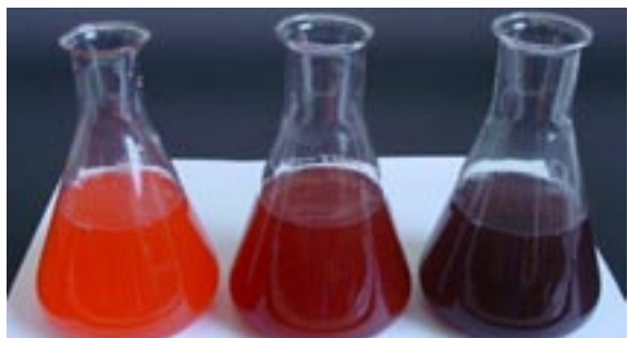
Figure 4 Red capsicum. Left flask: Before the endpoint, the solution retains its original colour. Centre flask: Once all the ascorbic acid has been oxidised, a slight excess of added iodine forms a dark complex with starch indicator giving a purple colour. This is the titration endpoint. Right flask: If a further mL or two of iodine were to be added after the endpoint, the solution would develop the dark purple colour shown here.
